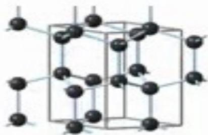
4-connected net Lonsdaleite ( P6_3/mmc ) Si(4f)
