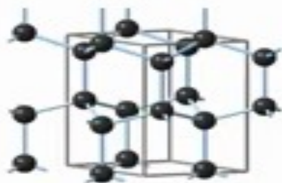
4-connected net Lonsdaleite ( P6_3/mmc ) Si(4f)
