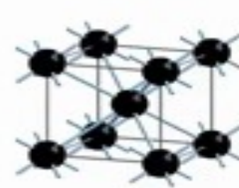
8-connected net Body-centered Cubic ( Im\bar{3}m )
