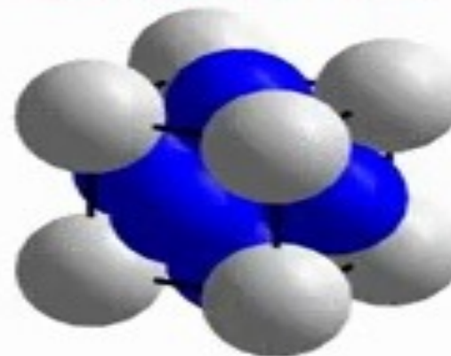
Cu 3 Au Structure Space Group: Pm\bar{3}m
