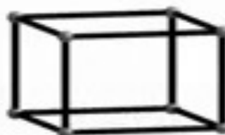
Monoclinic a \neq b \neq c \alpha = \gamma = 90^\circ, \beta \neq 90^\circ
